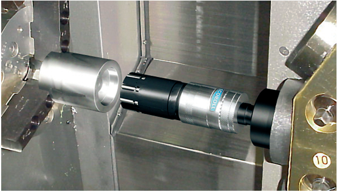
Type G roller burnishing tool on a CNC-controlled lathe.
