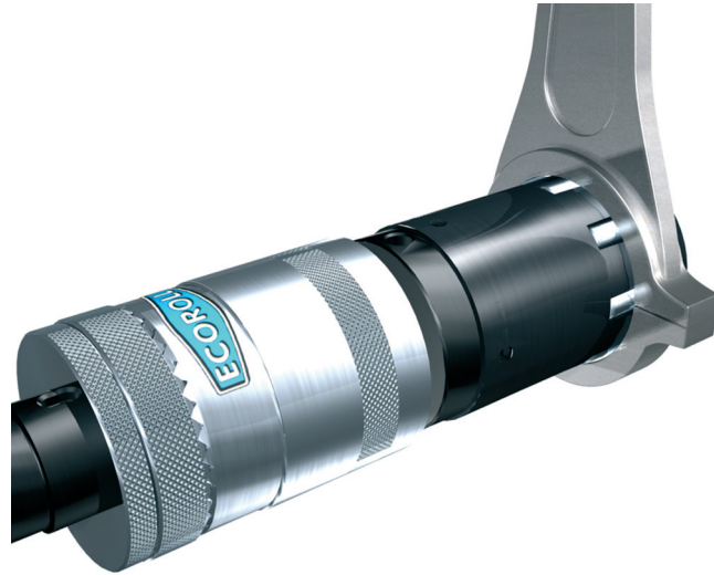
Machining a connecting rod with a Type G tool.
